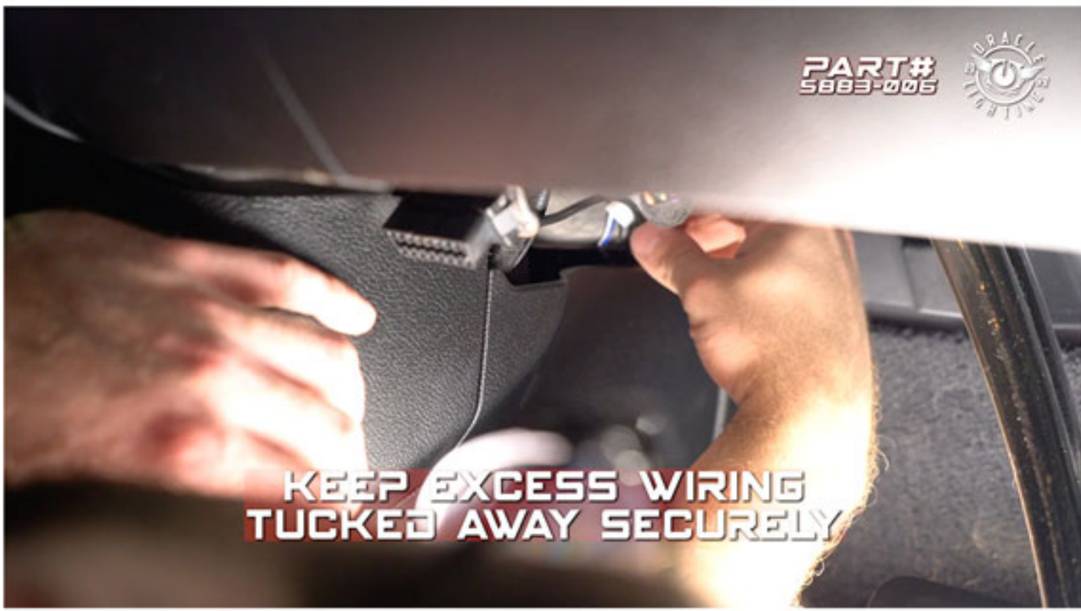
IN THE FOOTWELL CONNECT THE PLUG TO ON/OFF SWITCH
