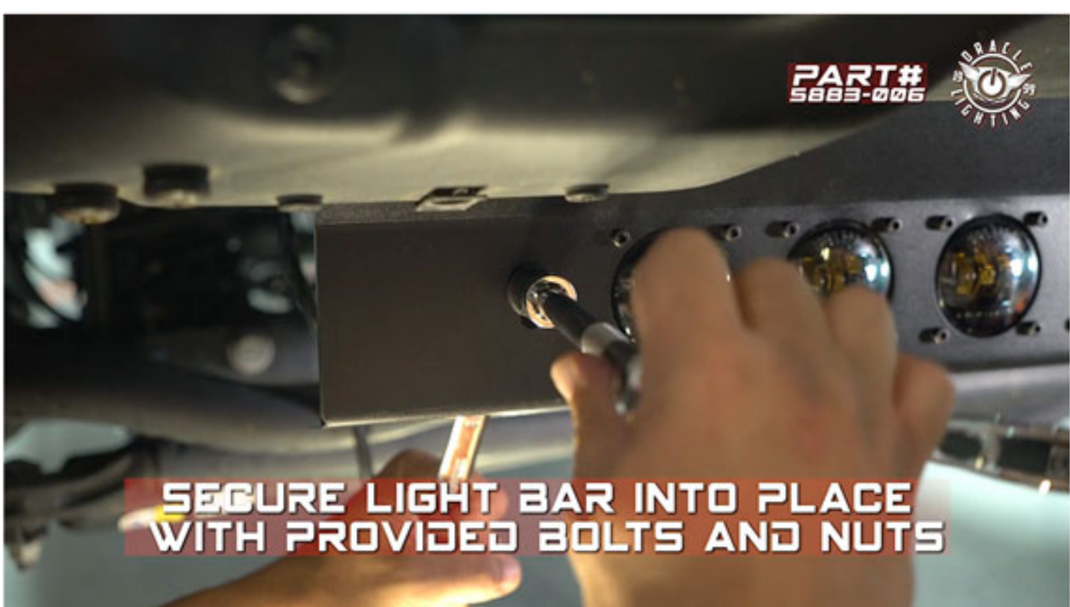
PLUG THE LIGHT BAR IN AND SECURE THE LIGHT BACK INTO PLACE
